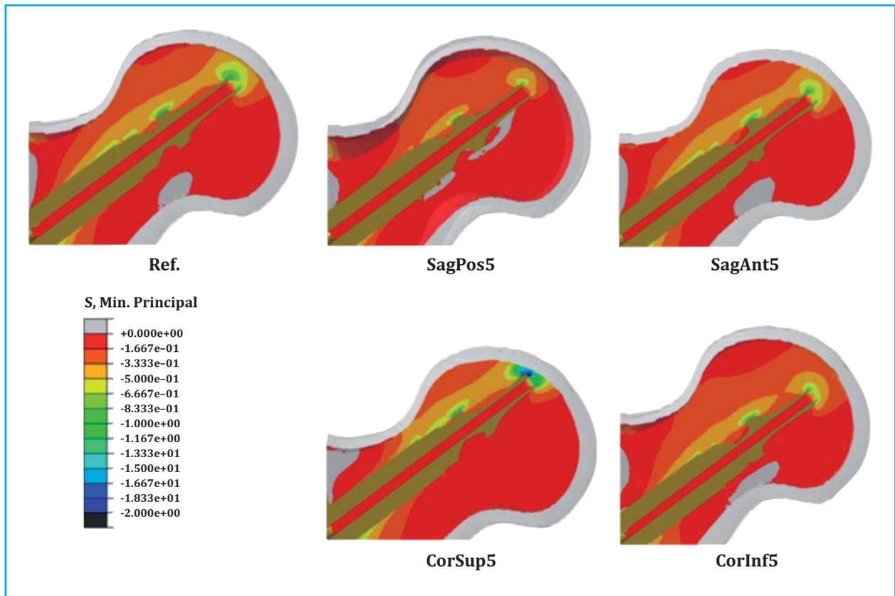
**Figure 10. Results obtained in the damaged femur model. A) Minimal major deformations in the trabecular bone. B) Global displacement field in the trabecular bone**
